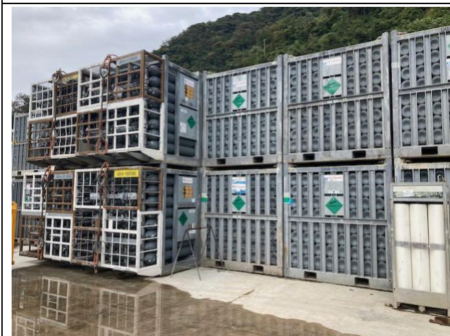
Photo 40: Gas bottles for divers stored at dam
